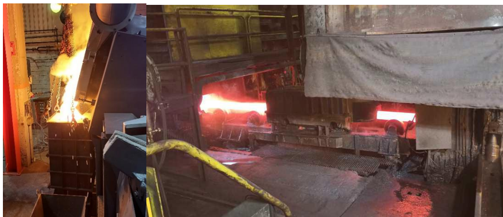
Preindustrial casting (left); Reduction of diameter in the stretch-reducing mill to final dimensions (right).
