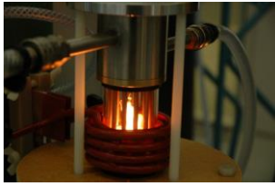
Vacuum levitation furnace Cu mold casting (rapid solidification) (1 Kg)
